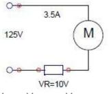
$$V_{red} = V_{motor} + V_{R}$$
